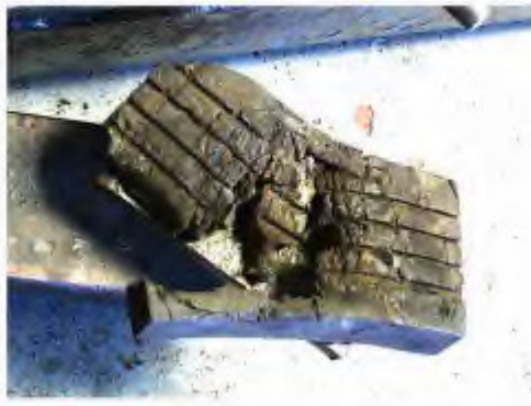
Examples of missing / defective / worn / and contaminated rubber pads
