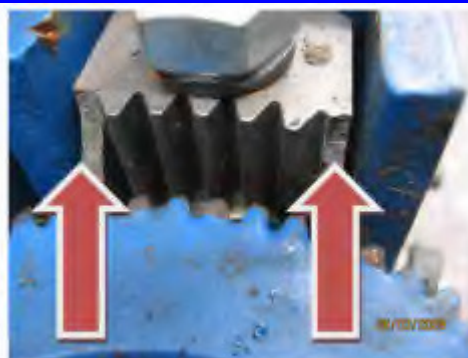
Damaged & Worn Teeth
